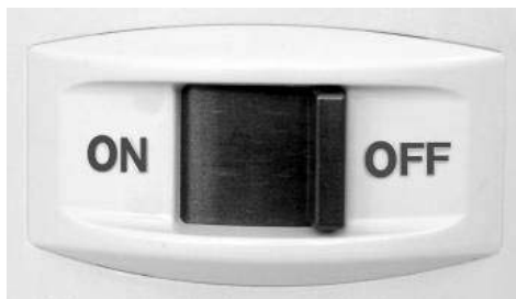
Unit OFF Compensator locked
